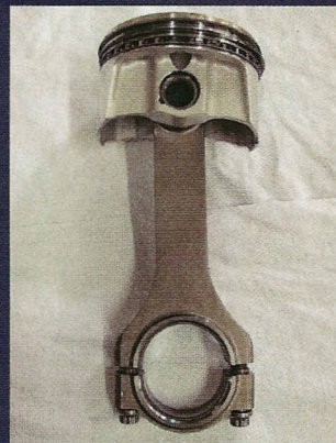
CP's Bullit line of forged pistons was utilized, as well as remanufactured Dyers forged H-beam connecting rods, resulting in a light-weight, strong rotating assembly.
