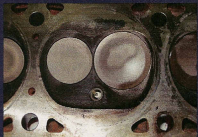
The real tricks employed by Schurbon Engine and Machine were in the RHS/Indy X cylinder heads. After completely porting
